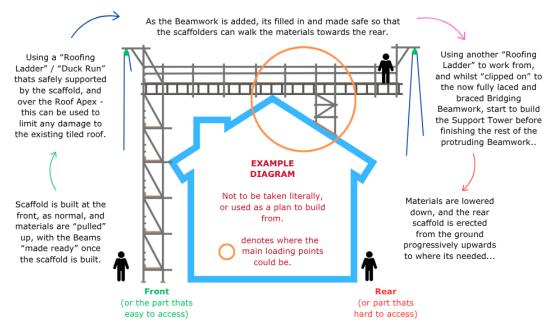
Now, these kinds of scaffolds would usually require a design to work from (as they do not come under TG guidance), due to the possible unknown loadings on the roofs apex, with this diagram to be used as **EXAMPLE ONLY** for those who might need an explanation of how they work. With our recommendation being to work in REVERSE of this during the dismantle process.
